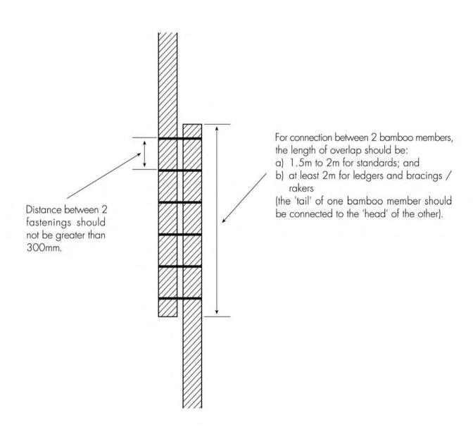
Figure 7: Single lift type truss-out bamboo scaffold (side elevation – not to scale)
