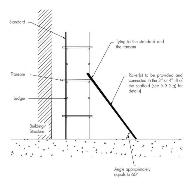
Figure 6: Showing the proper connection of bamboo members for bracings/rakers, ledgers, standards used in the erection of bamboo scaffold (not to scale)
