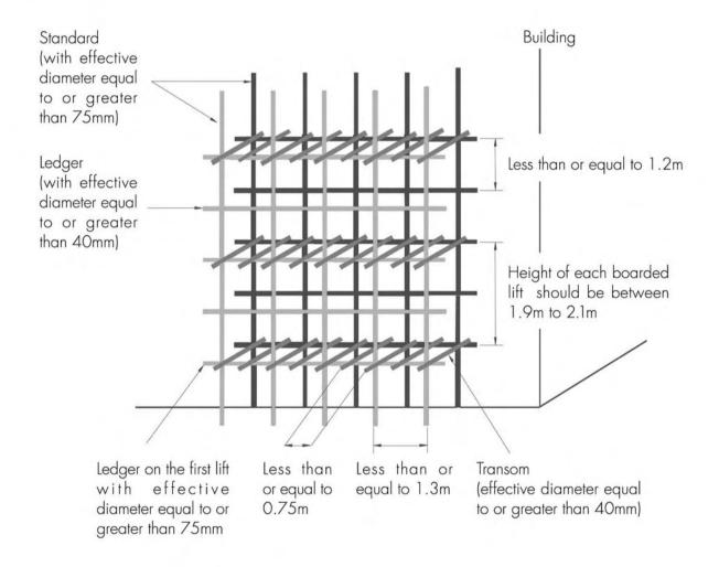
For all standards and the ledgers on the first lift of the scaffold, the wall thickness of these bamboo members should not be less than 10mm.
